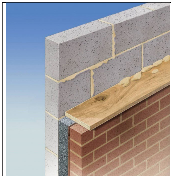
Figure 6 Use of a cavity board
